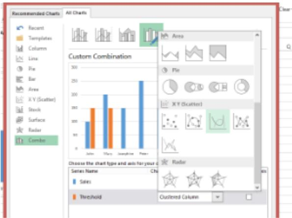
9. Choose the XY scatter type, scatter with smooth lines. Secondary X and Y axes should now appear
